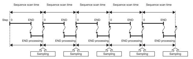
At the time of data sampling in each sequence scan, scan time increases due to transfer from a CPU module to a C intelligent function module.
